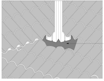
THE VALLEY METAL MUST LAP ONTO THE TILE OF THE COURSE BELOW THE ROOF TRANSITION FLASHING
