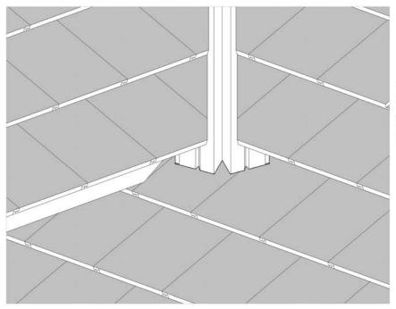
EXAMPLE FOR FLAT OR LOW PROFILE TILE THE VALLEY METAL MUST LAP ONTO THE TILE OF THE COURSE BELOW THE ROOF TRANSITION FLASHING
